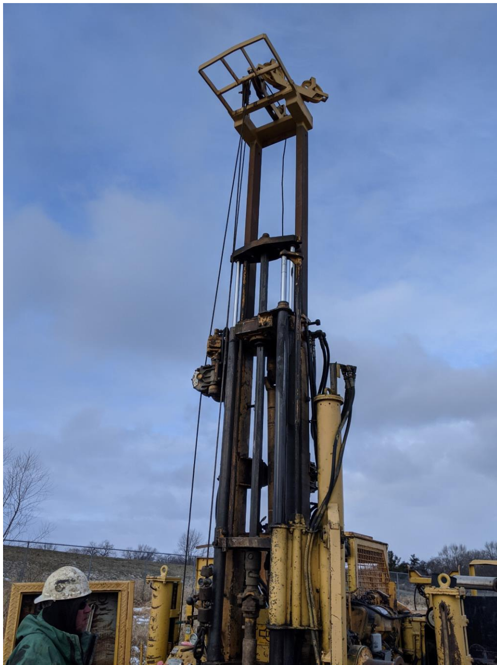
Left: Drill rig tower with winch on top to pull and lower center rod with center bit or split-spoon sampler, Kelly bar in center, automatic SPT hammer (yellow tube) on the right.
