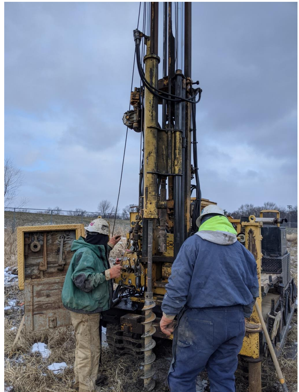
Right: SPT sampling with split-spoon sampler (not visible – at bottom of borehole) attached to center rod; note pink chalk marks on center rod at 6-in. centers: SPT sampling involves driving the sampler 18 in. below the (current) bottom of the borehole, and blows from the automatic SPT hammer required to advance the sampler 6 in. are being recorded on field logs. First, the sampler is seated 6 in. into the ground, and the total blows required to advance the sampler over the final 12 in. is designated the Standard Penetration Resistance (N-value) of the sample.
