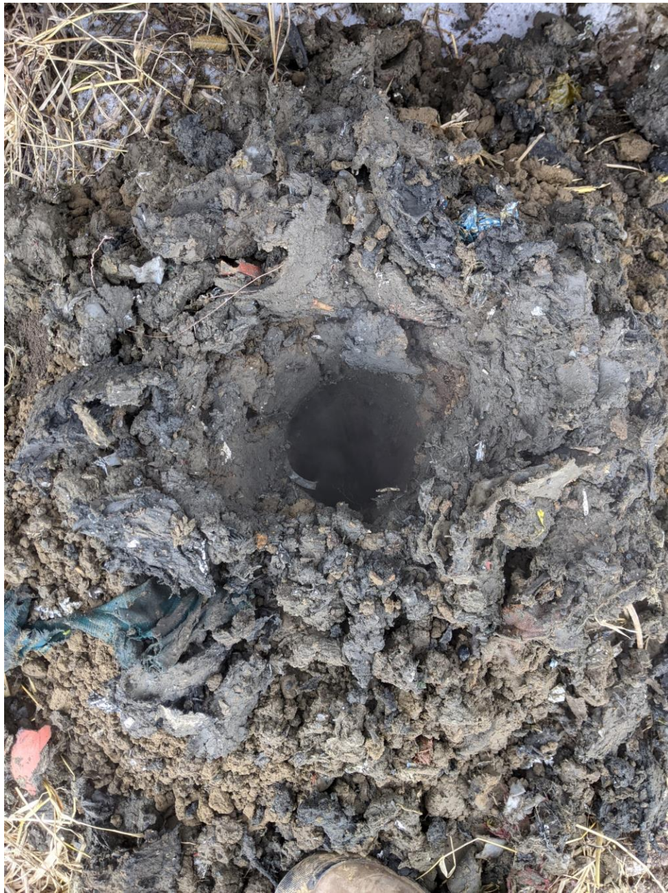
Left: B-3 upon completion of drilling after augers have been pulled; note warm air rising from the borehole and condensing.
