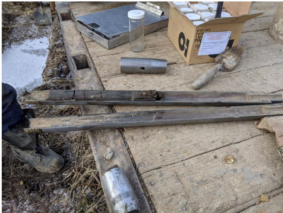
Upper left: Split-spoon barrel after sampling with extracted soil sample in it; tip of sampler at bottom of picture. Lower left: Box containing glass jars for soil samples and bags of bentonite chips.
