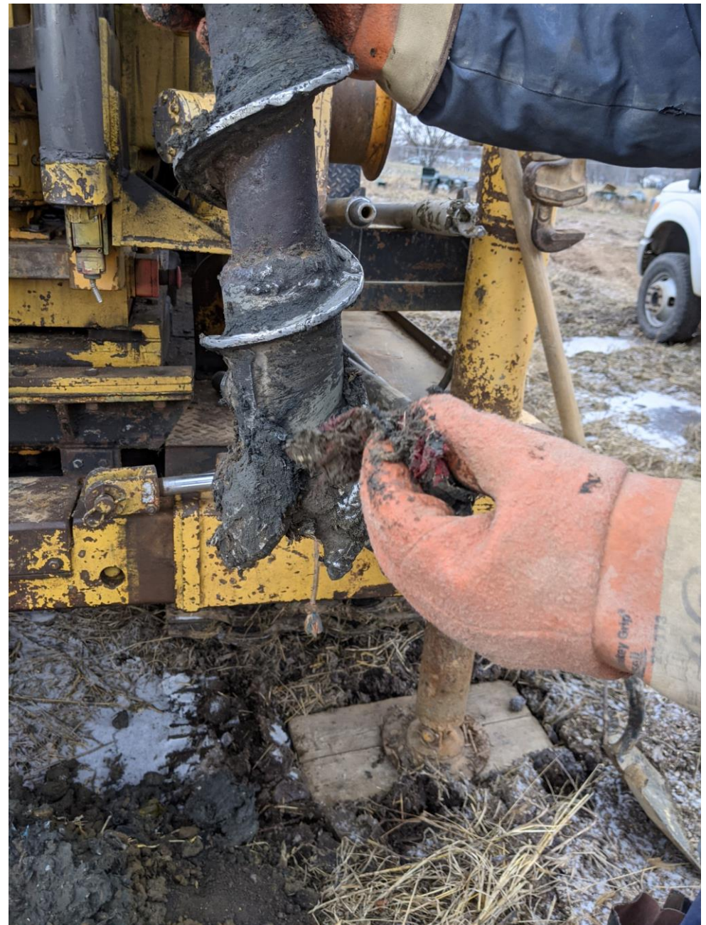
Right: Hollow-stem auger lead section pulled off hole after completing B-3; deleterious material wrapped around augers.
