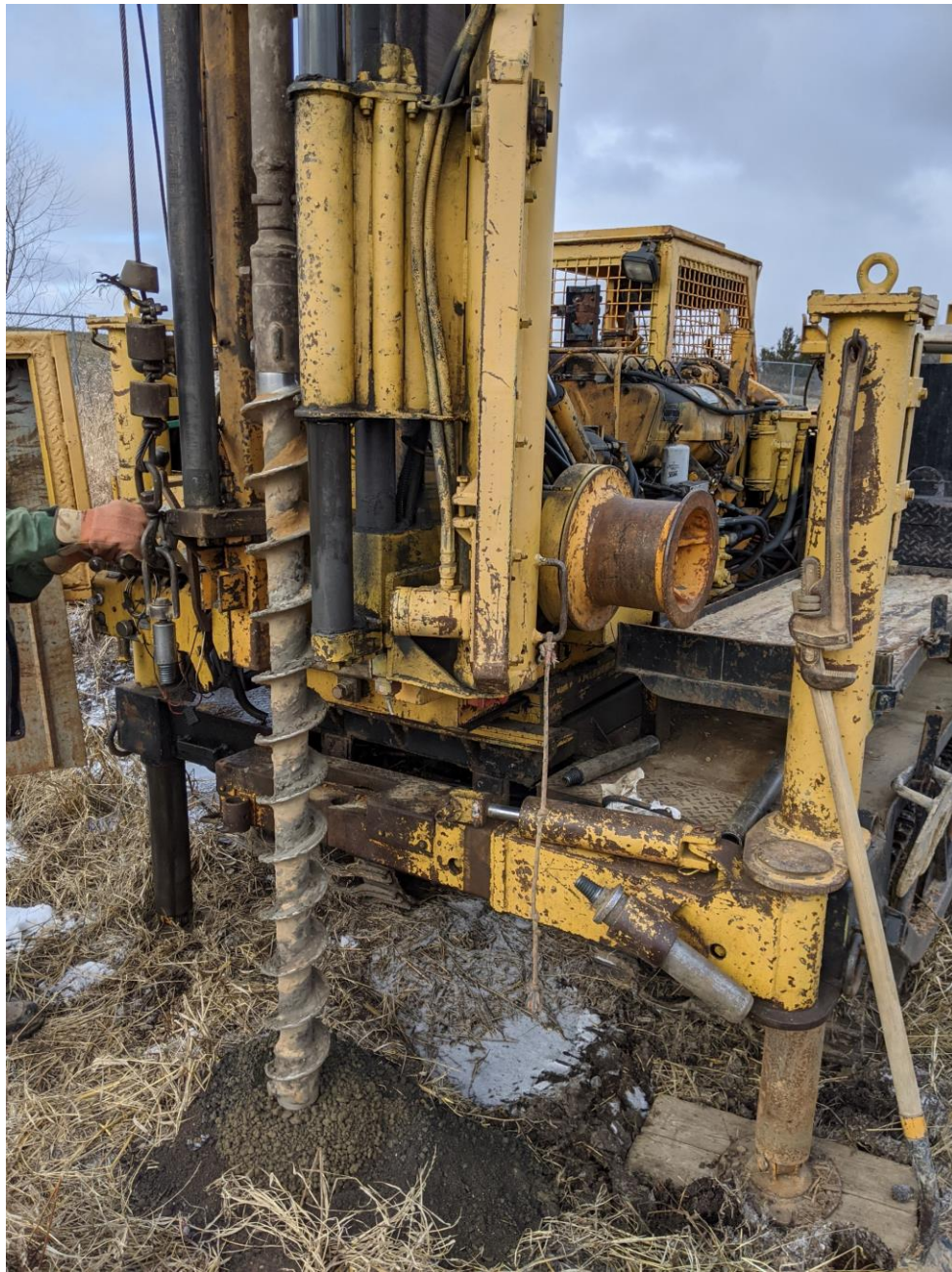
Left: Hollow-stem auger drilling with auger section attached to Kelly bar.
