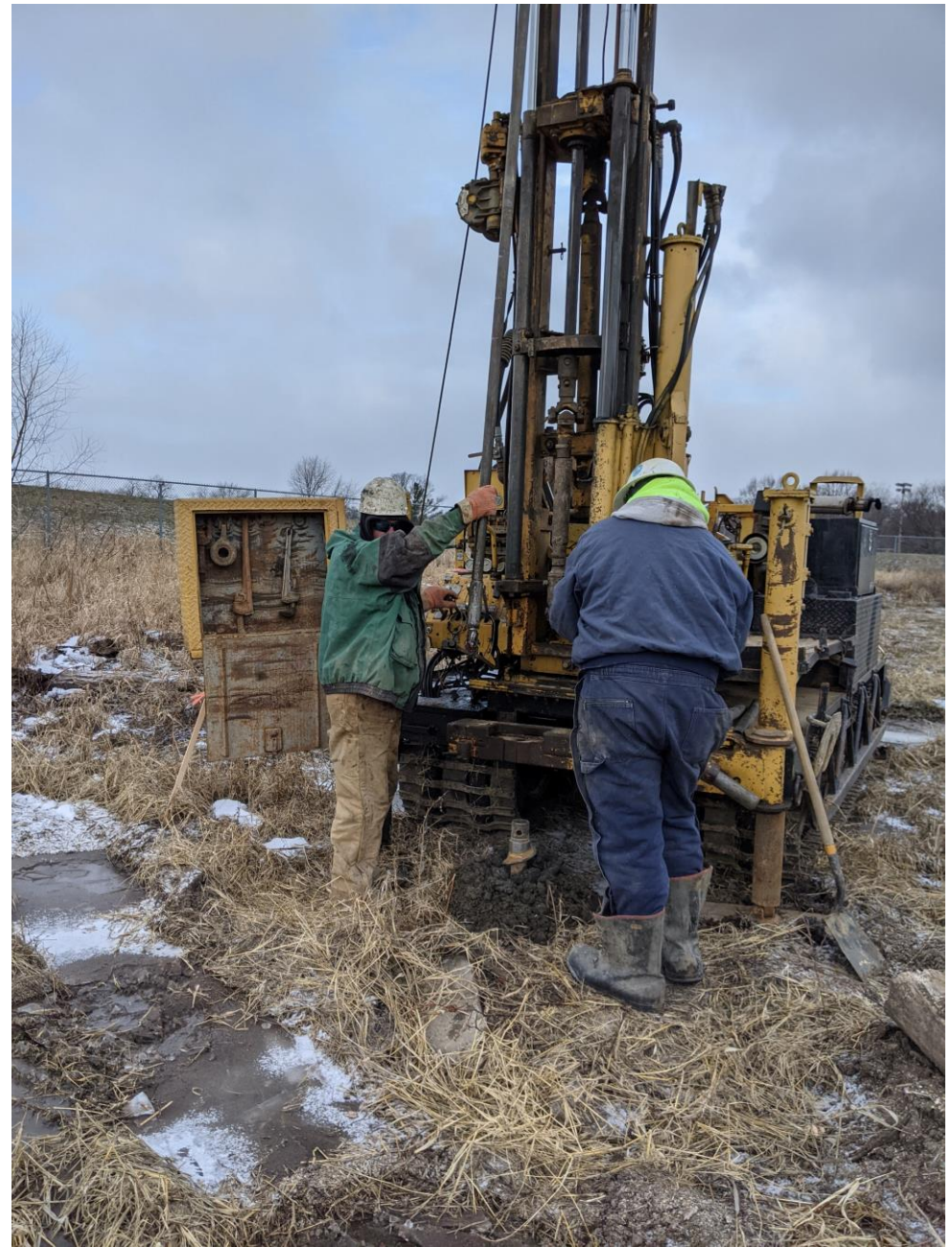
Right: Hollow-stem auger section sticking out of borehole, uncoupled from the drill rig's Kelly bar; center rod with attached center bit being pulled out of the augers to prepare for sampling.
