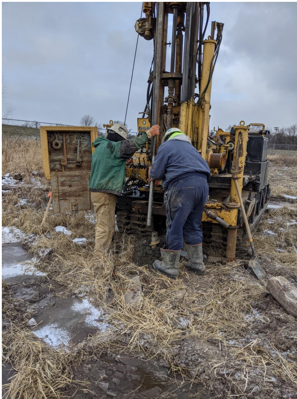
Left: Split-spoon sampler being attached to center rod, which will be lowered into the borehole through the hollow-stem auger sections to sample the borehole bottom.
