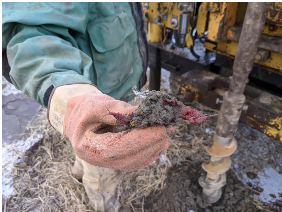
Upper left: Deleterious material (fabric shreds) intermixed with soil.
