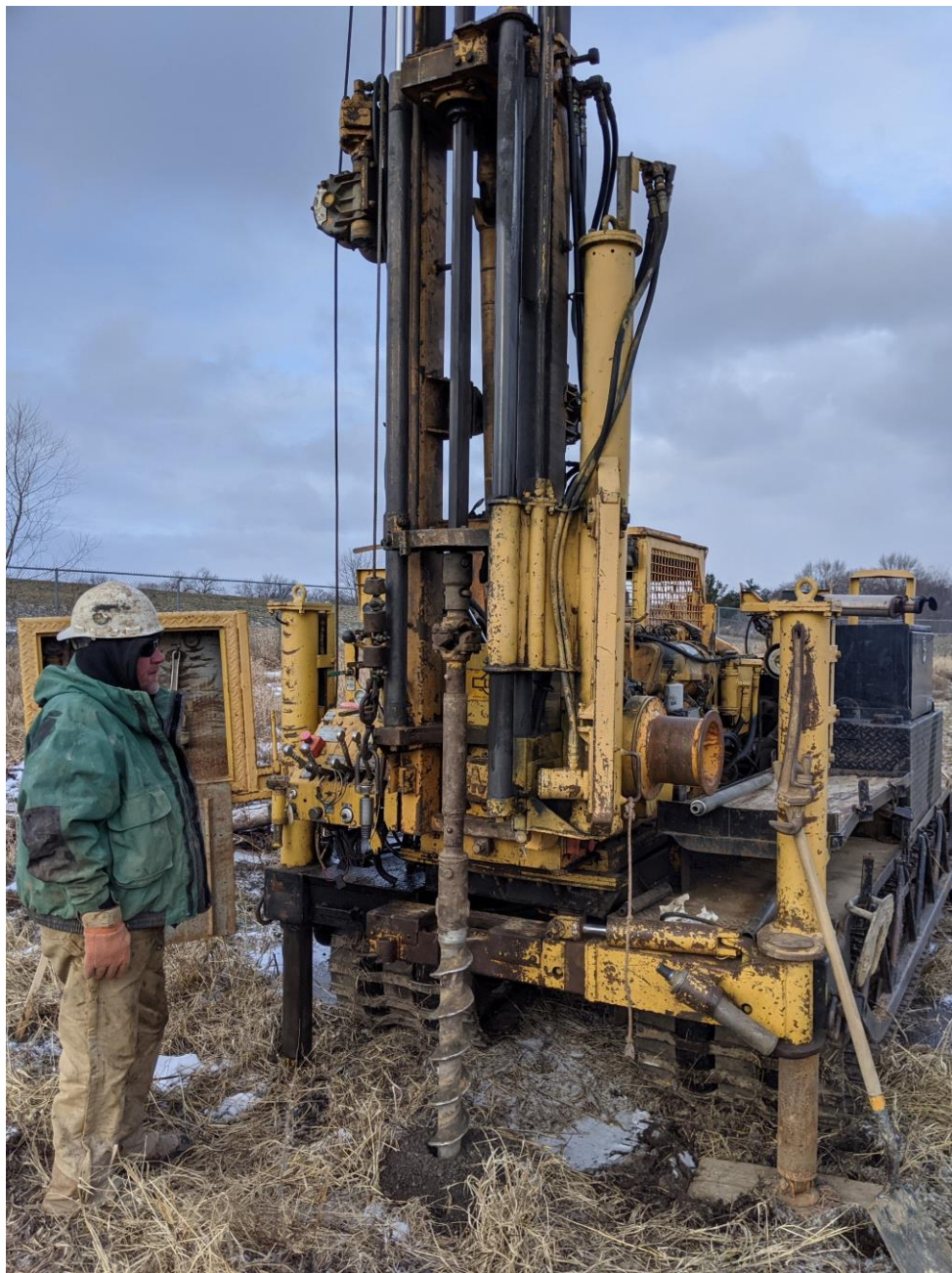
Left: Hollow-stem auger drilling with auger cuttings accumulating around the borehole.
