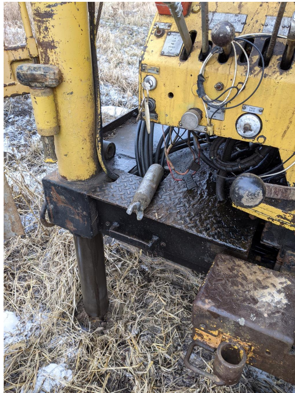
Right: Detached center bit during SPT sampling.
