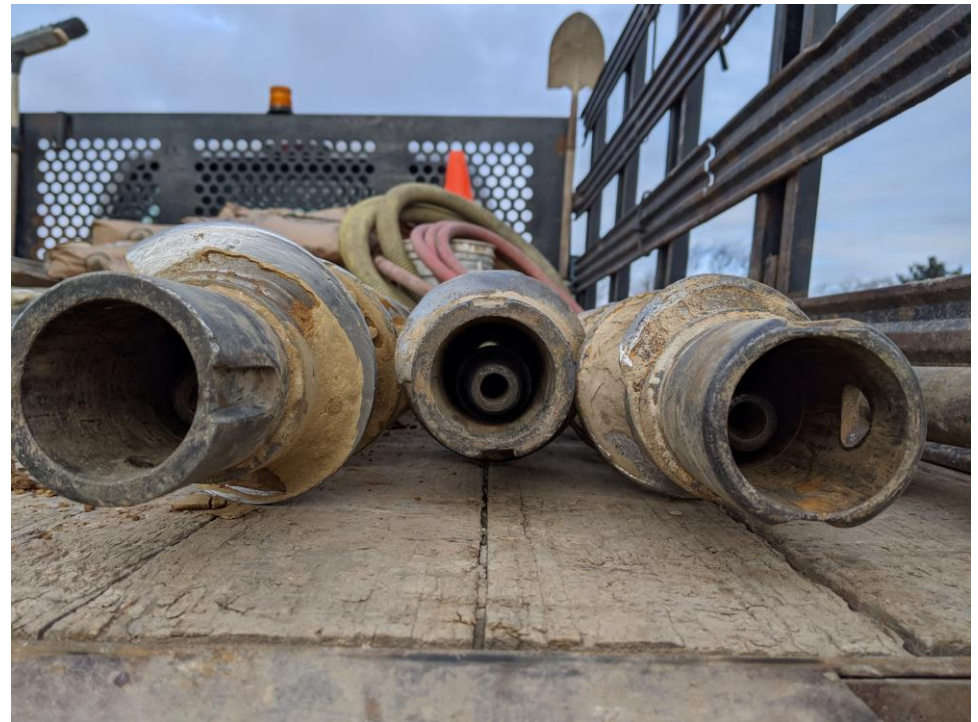
Lower right: 2-1/4 in. hollow-stem augers with center rod.
